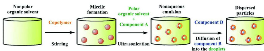
Figure 9. Schematic description of the polymerization in nonaqueous emulsion. (see color insert)
